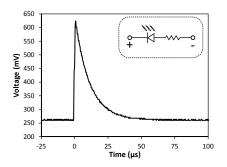
Single photon detection with an actively quenched light emitting diode
