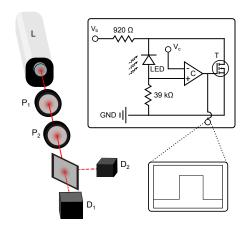
Single photon detection with an actively quenched light emitting diode
