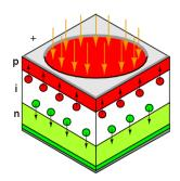
Single photon detection with an actively quenched light emitting diode
